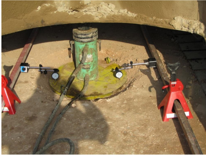
Plate (3): Plate Bearing Test for Location of Tank DO Set 7
