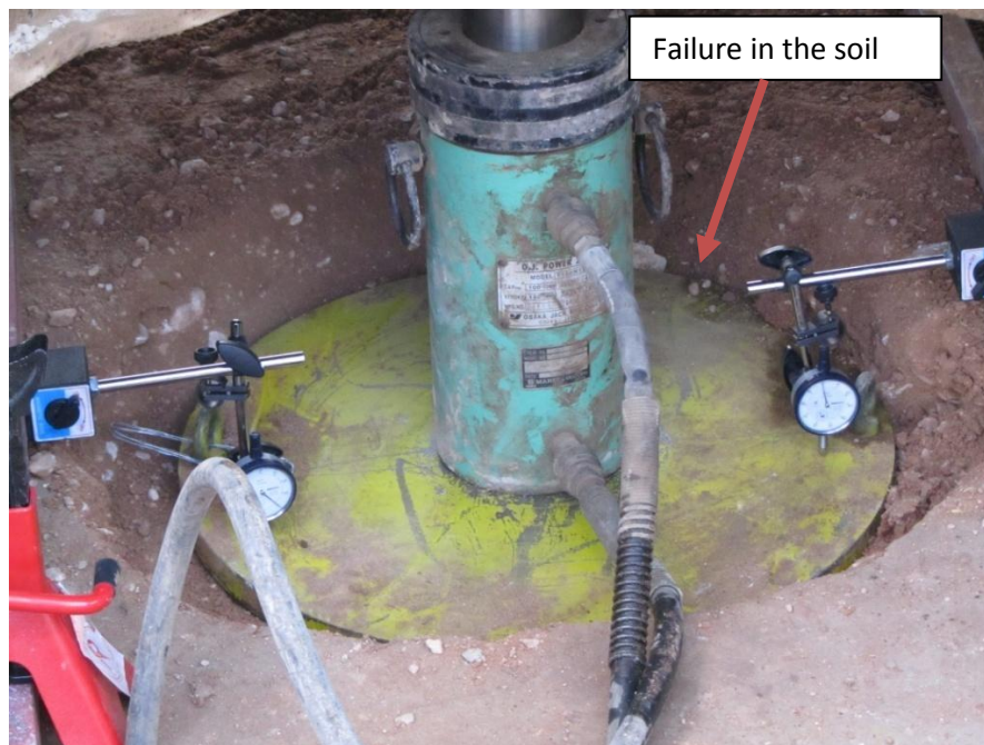
Plate (4): Plate Bearing Test for Location of MDU 4 Set 6
